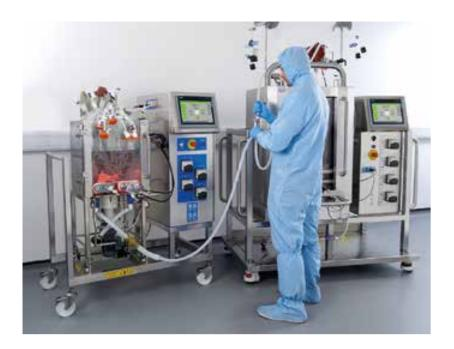
Above: This bioreactors photograph is reflective of the specialist manufacturing equipment VMIC purchased and had installed in Virtual VMIC, the rapid deployment centre. Includes Allegro™ STR bioreactors 50 L and 200 L from Pall corporation.
